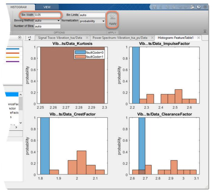
At this resolution, both CrestFactor and ImpulseFactor appear to completely separate healthy from faulty data. ClearanceFactor still has some mixed data, but to a lesser degree than with the larger bin width. Kurtosis had a smaller bin width of 0.002 with the auto bin width setting. Changing the bin width to 0.05 results in a single bin that contains all the Kurtosis data.
