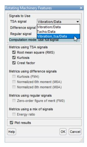
Other feature choices in the dialog box use the filtered TSA difference and regular signals as a source. This example does not use the difference and regular signal-based features because computation for those signals assumes common shaft speed.
