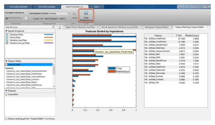
The Bhattacharyya technique yields results that are similar to, but not identical to, the T-Test results. The highest ranking feature is PeakValue from the Signal Statistics set.
