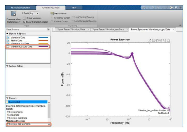
The power spectrum processing results in a new variable, Vibration\_tsa\_ps. The associated icon represents a linear model, consistent with the AR model default in the power spectrum dialog box.
