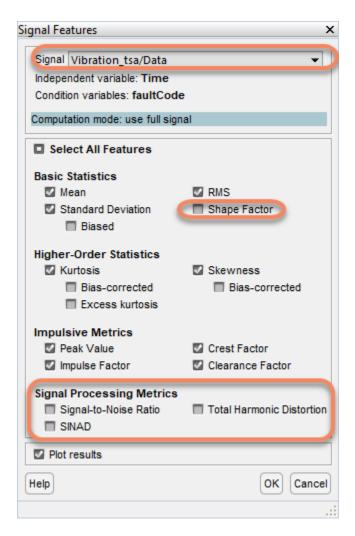
For every selected feature, the app computes a value for each ensemble member and displays the results in a histogram. Each histogram contains bins containing the number of feature values which fall within the bin range. The **Histogram** tab displays parameters that determine the content and resolution of the histograms.
