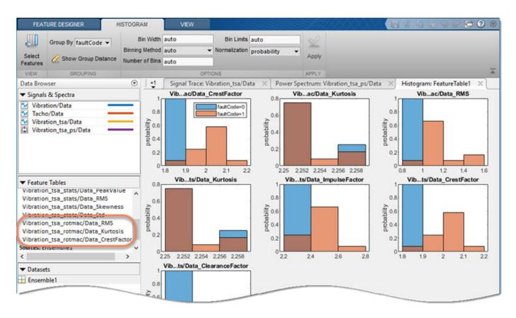
The app automatically adds the new features to the feature table and the **Select Features** list, and plots the new histograms at the top of the histogram display. CrestFactor and Kurtosis histograms are essentially the same whether they were computed as signal features or rotating machinery features, since both computations used the TSA signal as a source.
